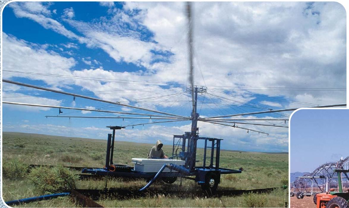
*(Above) Under the rotating boom rainfall simulator he operates, hydraulic engineer Gary Frasier gathers information on soil infiltration and water runoff. (Right) Soil core samples are withdrawn from a field near Fort Collins, Colorado, by technician Mike Murphy and soil scientist Laj Ahuja. Photo credit Scott Bauer, U.S. Department of Agriculture.*
