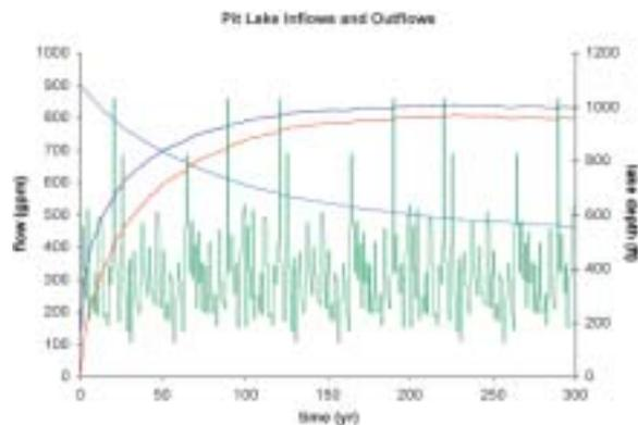
Figure 1: green line: surface water inflows (gpm); light blue line: groundwater inflows (gpm); red line: evaporation (gpm); dark blue line: pit lake water depth (ft).
