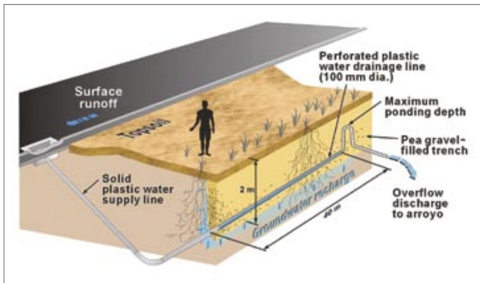
Schematic diagram of a typical siphon-infiltration trench. The infiltration trench can be applied to most locations where diversion of surface water to the subsurface is desirable.
