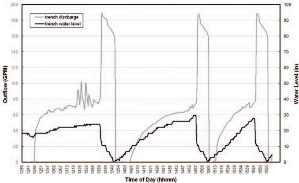
Flow rates under siphoning and non-siphoning conditions. When water levels rise to an engineered height, the siphon is actuated. The three peaks in flow rate correspond to three separate siphoning events. After the trench drains, the siphon is broken, and water levels begin to rise again. Infiltration into the surrounding soil occurs continuously.
