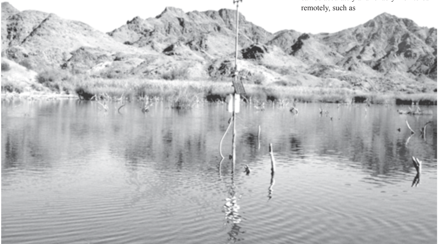
Water quality and weather monitoring at Lake Havasu National Wildlife Refuge near Needles, California. Photo courtesy of Intermountain Environmental, Inc.
