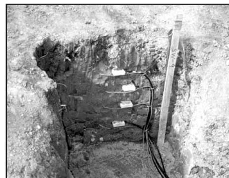
Installation of automated HDS and water content reflectometer arrays in a nuclear repository clay cover.
