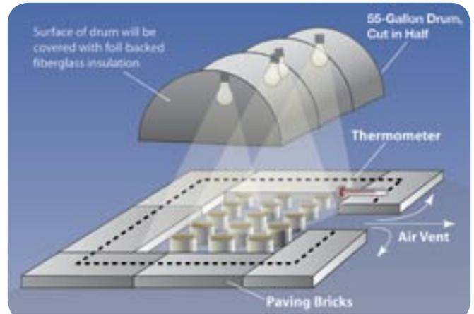
Schematic of the GLOBE SMC light-bulb oven.
