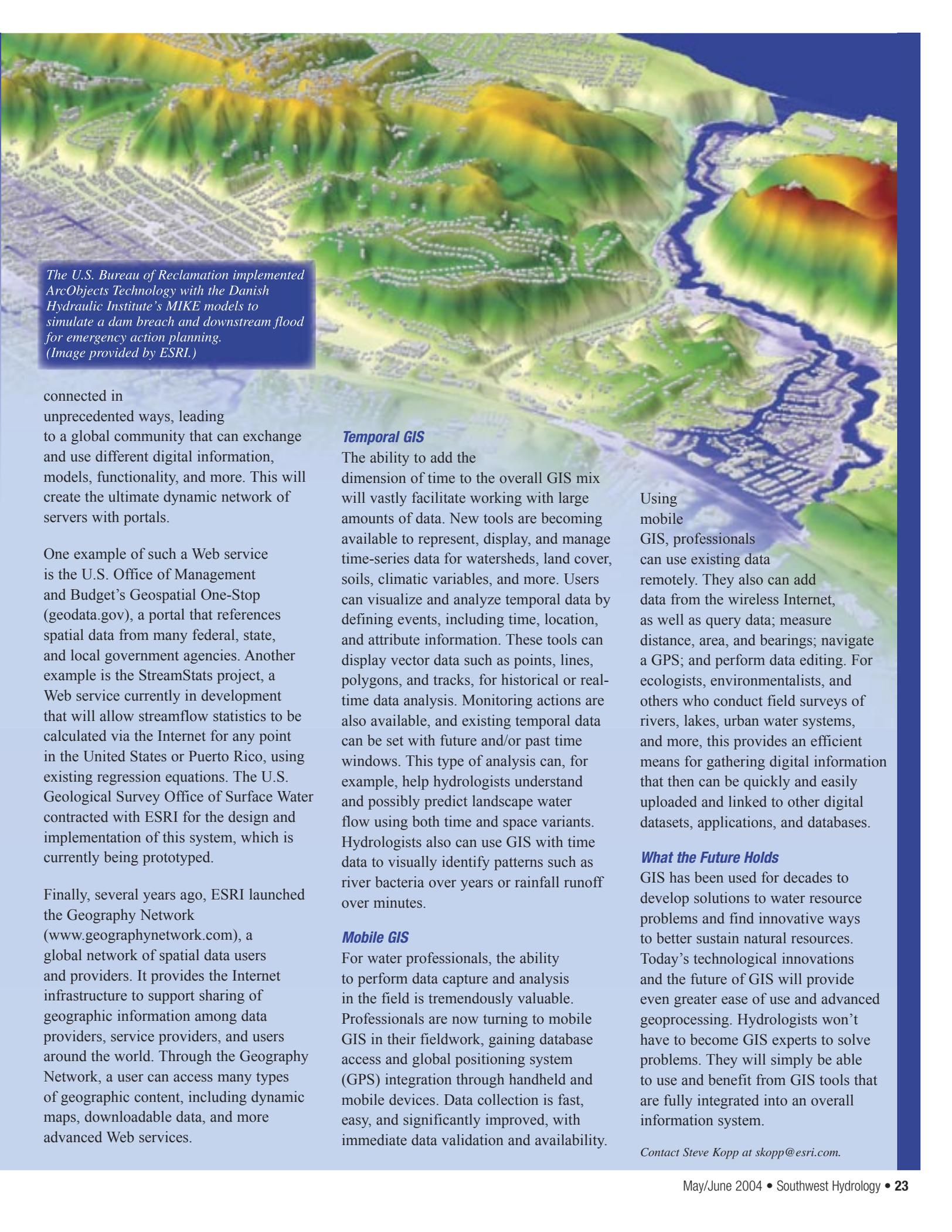
*The U.S. Bureau of Reclamation implemented ArcObjects Technology with the Danish Hydraulic Institute's MIKE models to simulate a dam breach and downstream flood for emergency action planning. (Image provided by ESRI.)*
