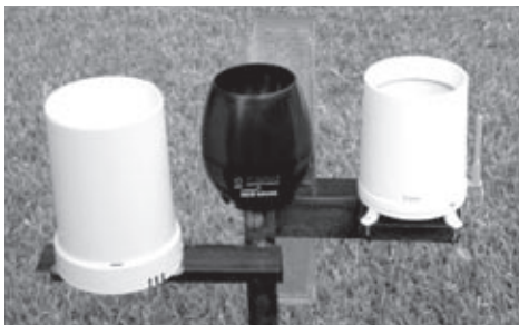
From left, the LaCrosse, Torrent, and Oregon Scientific digital gauges, and Tru-Chek (in back) set up for testing.
