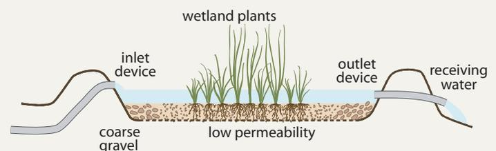
*Profile of a typical free-water surface wetland.*
