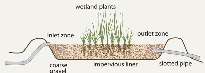
*Profile of a vegetated gravel or subsurface flow wetland.*
