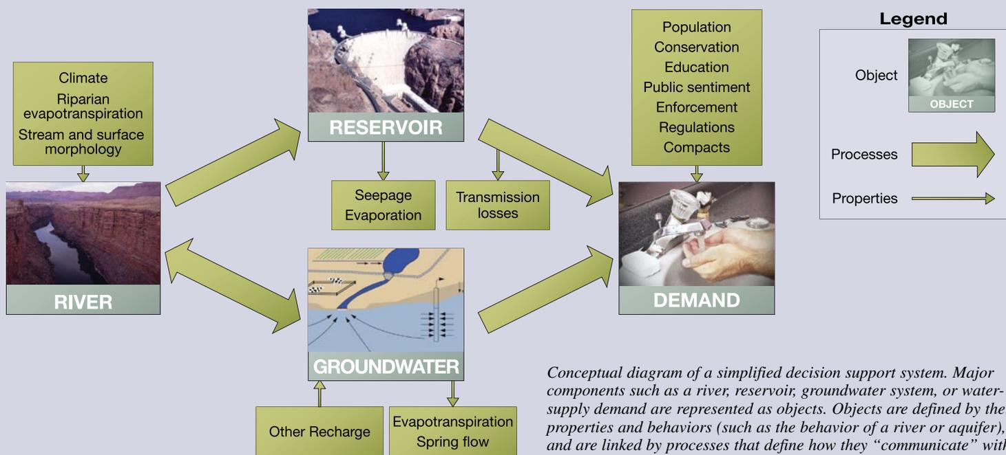
Conceptual diagram of a simplified decision support system. Major components such as a river, reservoir, groundwater system, or water-supply demand are represented as objects. Objects are defined by their properties and behaviors (such as the behavior of a river or aquifer), and are linked by processes that define how they "communicate" with other objects (such as groundwater/surface water interaction).
