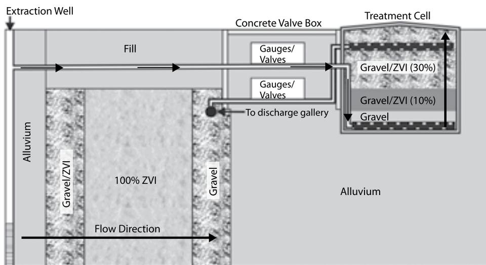
Contaminated groundwater at the Monticello site is now extracted from a well upgradient of the PRB and routed to an adjacent ex-situ treatment cell.
