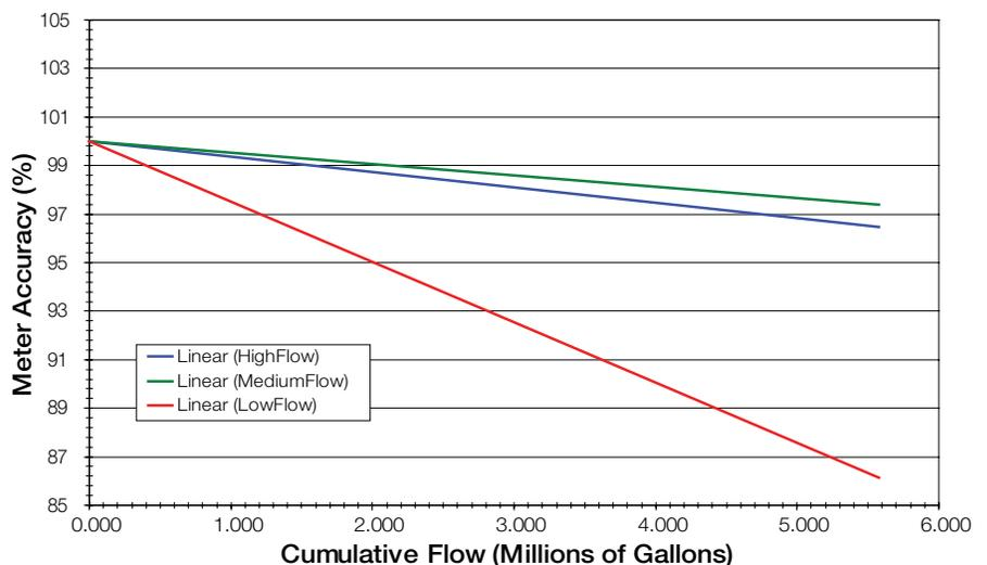
Accuracy of Metro Water's 3/4-inch meters as a function of flow rate and cumulative volume metered.
