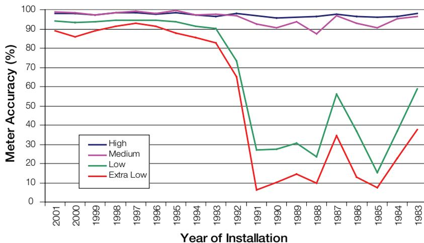
Accuracy of Phoenix Water's 3/4-inch meters as a function of flow rate and year installed.
