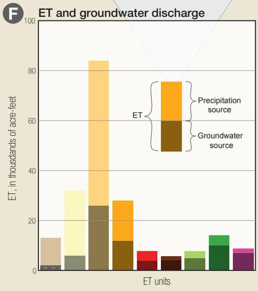
Conceptualization of the ET units and the groundwater discharge estimation process for Spring Valley.
