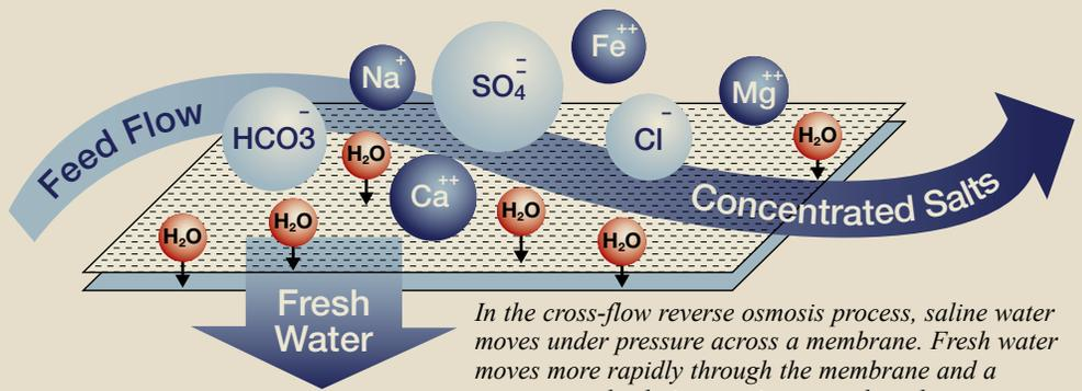
impeded the use of desalination, but recent technological advancements such as high-efficiency pumps, energy-recovery devices, and higher-productivity membranes are now making desalination more viable.
