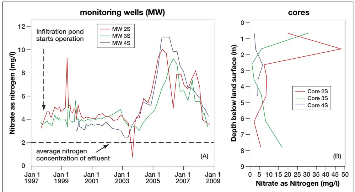
(left) Eight years after an infiltration pond began operating, a pulse of high-nitrate groundwater was observed in monitoring wells. (right) Nitrogen concentrations in sediment samples taken from the same wells are highest in the upper 10 feet.
