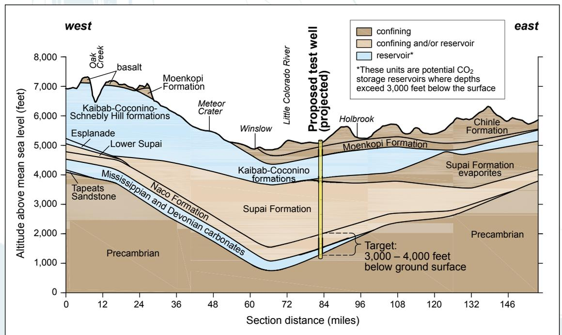
East-west regional schematic geologic cross-section of the WESTCARB CO<sub>2</sub> sequestration pilot project.
