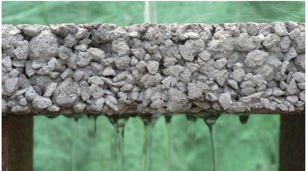
*Pervious cement manufactured by TecEco of Australia (image courtesy of John Harrison).*
